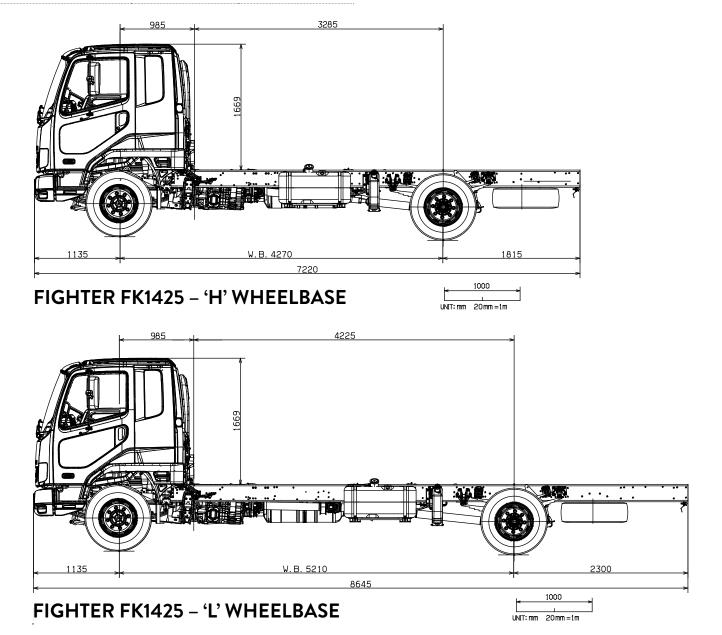
Scale = 1:50 (20mm = 1 metre). This scale is accurate when used on the original spec sheet, be aware that enlarging these illustrations can alter the scale and cause incorrect measurements. Fuso New Zealand and its authorised dealers always recommend customers seek professional advice from independent sources before commencing any engineering activities.
